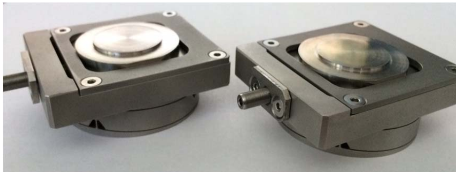
Figure 7 – Grating Mosaic Design with Adjustable Shims
