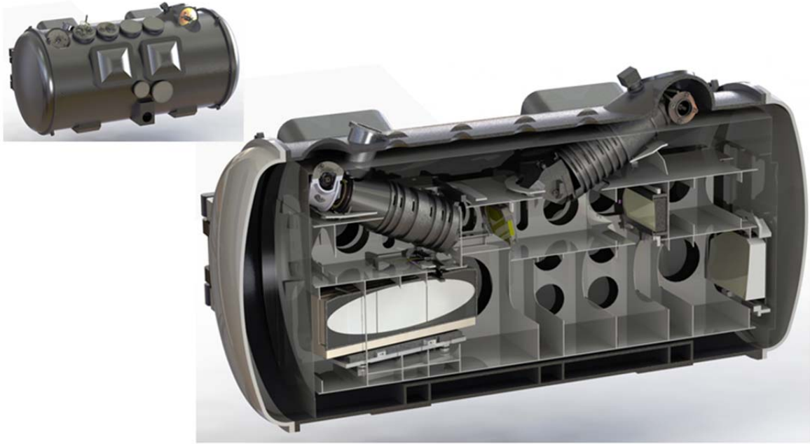
Figure 9 – Cylindrical Vacuum Chamber Concept with Section View
