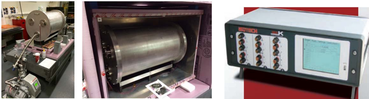
Figure 11 – Thermal Prototype Set-Up Showing our Scaled Vacuum Chamber, Thermal Panel Assemblies and Isotech Precision Measurement Electronics
